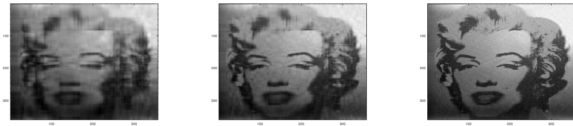
Figure 1.9. Successive SVD approximations of Andy Warhol's painting, Marilyn Diptych (~1960), with k = 10, 20, 40 rank-one updates.
