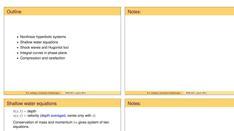
mass flux = hu, momentum flux = (hu)u + p where p = hydrostatic pressure
