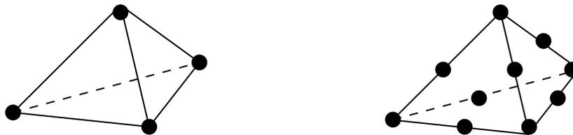
**Figure 9.18.** Finite element spaces in 3D. Left diagram:  $T_1(K)$  (linear) in  $H^1 \cap C^0$  whose degree of the freedom is 4; Right diagram:  $T_2(K)$  (quadratic) in  $H^1 \cap C^0$  whose degree of the freedom is 10.
